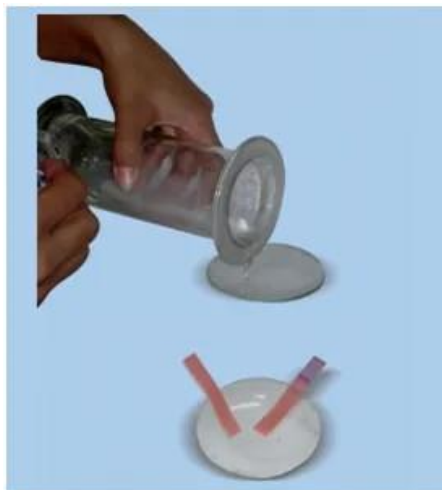
Testing of Solution with Litmus paper
